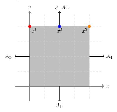
In this situation is clear that  $x^1$ ,  $x^3$ , and all solutions lying on the line between these two points are optimal. The simplex algorithm will return either  $x^1$  or  $x^3$  (and may switch if you change parameters). The barrier algorithm (without crossover) will return  $x^2$ . These solutions are all correct; the problem as stated has no reason to prefer one over the other. If you do have a preference, you'll need to state it in your objective function.
